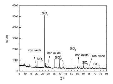
Fig. 3 The XRD mineral phase analysis spectrogram of magnetite
