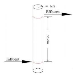
Fig. 1 Experimental device for the column test
