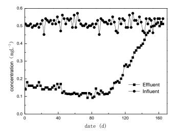
Fig. 5 Phosphorus concentrations in the effluents from the magnetite columns
