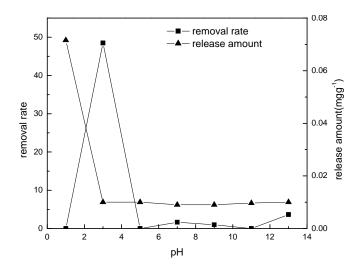
Fig. 4 Effect of pH on adsorption efficiency of phosphate by magnetite
