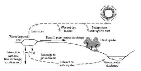
Fig. 3 Some fate and transport processes in subsurface and atmospheric environment
