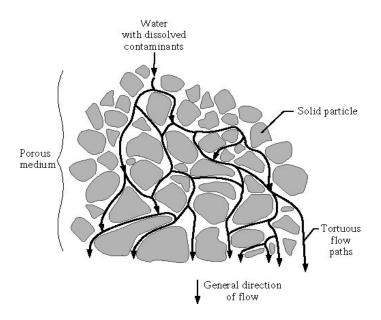
Fig. 2 Schematic of mechanical dispersion
