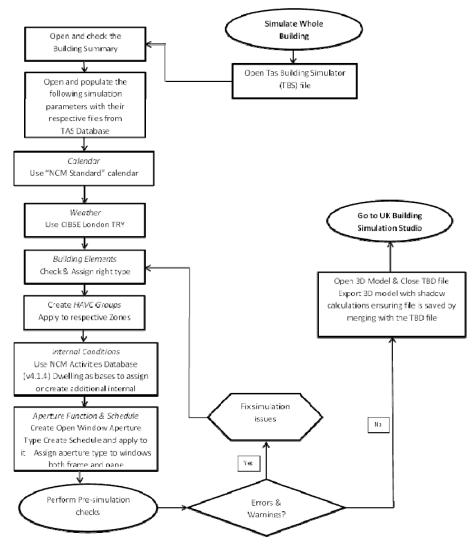
Fig. 7 Thermal simulation process
