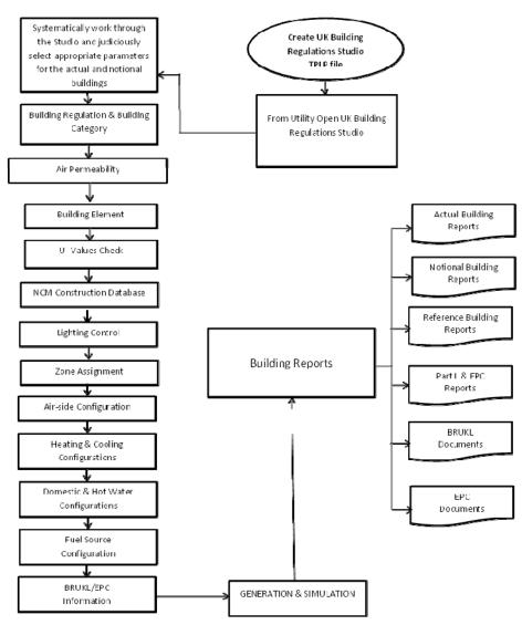
Fig. 8 UK building regulation studio simulation
