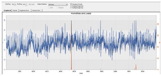
Fig. 23 Humidity and load analysis - 2080s high try all zones
