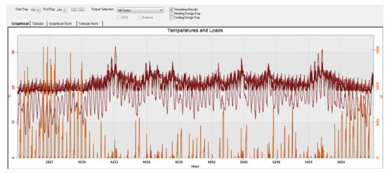
Fig. 18 Temperature and loads analysis - current weather data all zones
