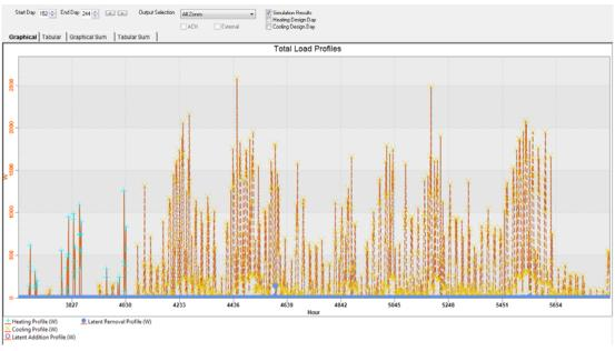
Fig. 25 Total load profiles analysis - 2080s high try all zones
