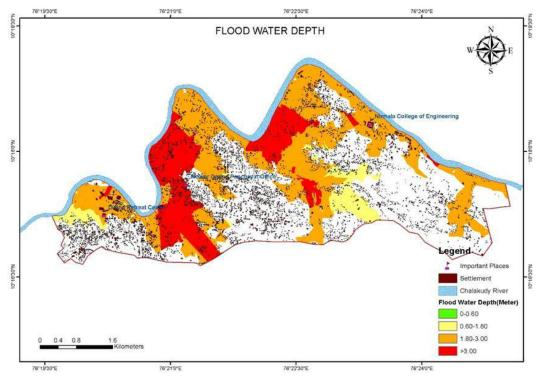
Fig. 6 Floodwater depth classification map
