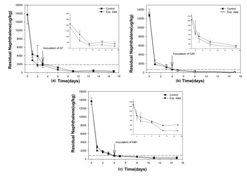
Fig. 4 Residual naphthalene in Heukyeumji soil in an air sparging system. Arrow indicates the point of strain inoculation. Liquid phase naphthalene was not detected below the dashed line. Flow rate: 60 ml/min; control: air sparging only. The error bars represent standard deviation (n = 3)
