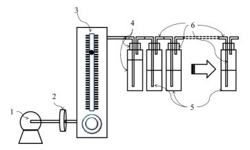
Fig. 1 Experimental apparatus for air sparging system (1) Air blower; 2 0.2  $\mu$ m Filter; 3 Flow meter; 4 Humidifier; 5 Soil slurry vials; 6 Air flow tubes)
