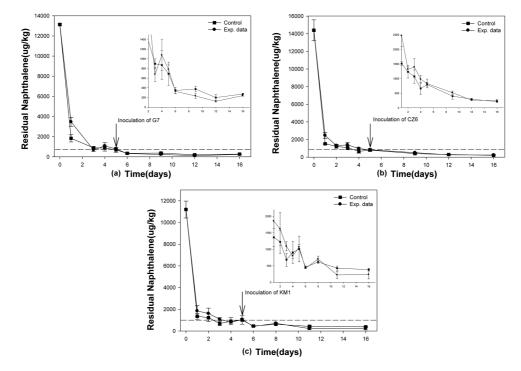
Fig. 5 Residual naphthalene in Jangseong soil in an air sparging system. Arrow indicates the point of strain inoculation. Liquid phase naphthalene was not detected below the dashed line; flow rate: 60 ml/min; control: air sparging only. The error bars represent standard deviation (n = 3)
