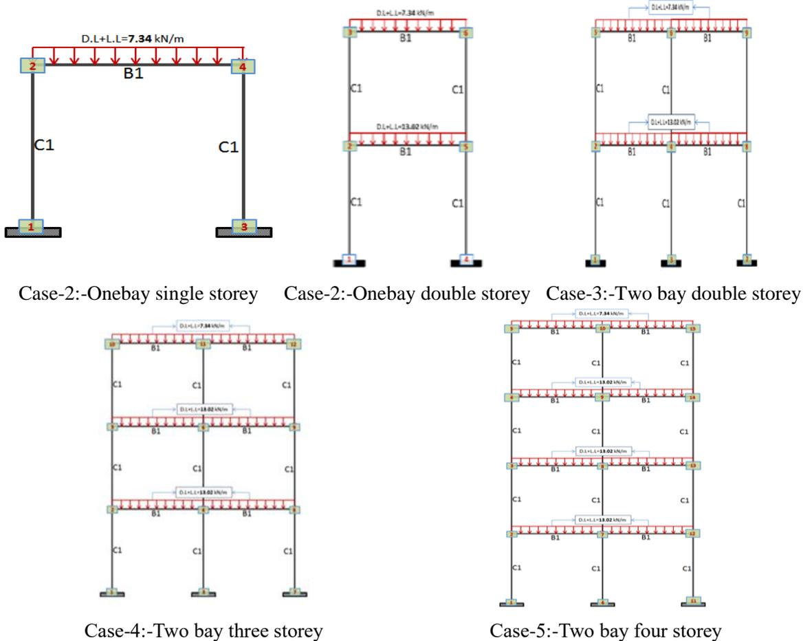
Fig. 1 Different types of 2D reinforced concrete frames considered for Analysis
