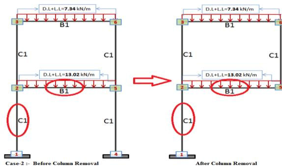
Fig. 2 Location of elements of one bay single storey 2D Reinforced Concrete Framed Structure for Analysis, Red Color Circles specify the structural elements, the effect of column removal are examined on these elements
