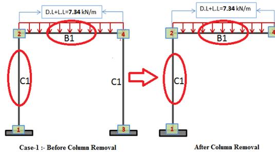
Fig. 3 Location of elements of one bay double storey 2D Reinforced Concrete Framed Structure for Analysis, Red Color Circles specify the structural elements, the effect of column removal are examined on these elements
