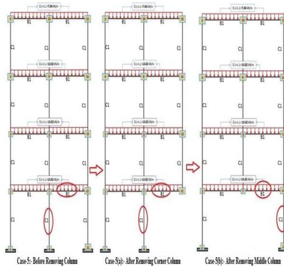
Fig. 6 Shows the Location of elements of two bay four storey 2D Reinforced Concrete Framed Structure which are to be Analyzed, Red Color Circles specify the structural elements, the effect of column removal are examined on these elements
