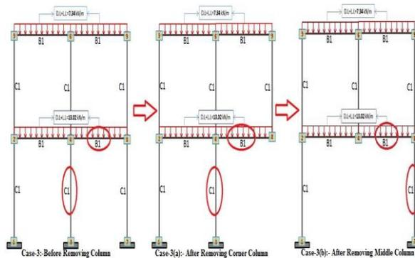
Fig. 4 Location of elements of two bay double Storey 2D Reinforced Concrete Framed Structure for Analysis, Red Color Circles specify the structural elements, the effect of column removal are examined on these elements
