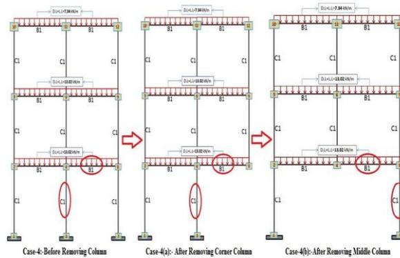
Fig. 5 Shows the Location of elements of two bay three storey 2D Reinforced Concrete Framed Structure which are to be Analyzed, Red Color Circles specify the structural elements, the effect of column removal are examined on these elements
