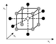
Fig. 3 Central composite design for three factors experiment
