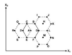
Fig. 1 Hexagonal Doehlert two factors design with three possible displacements in the experimental space
