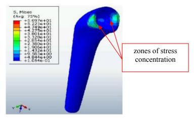
Fig. 5 Distribution of Von Mises stresses in orthopedic cement.
