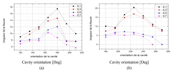
Fig. 14 Evolution of the maximum crack length for different cavity shapes and inclinations in both cases: (a) Position 1 and (b) Position
