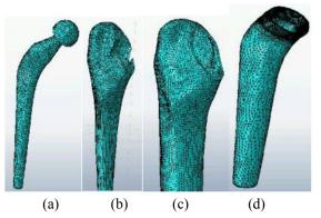
Fig. 4 Mesh of all THR components: (a) implant, (b) sponge bone, (c) cortical bone and (d) cement
