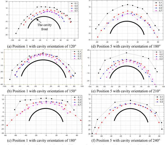
Fig. 12 Evolution of the crack front for different cavity shapes for positions 1 and 5 of the distal zone
