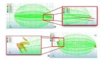
Fig. 11 Illustration of cracks for different cavity shapes in the distal area: (a) Position 1, (b) Position 5
