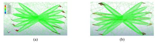
Fig. 13 Illustration of the crack initiation for different cavity inclinations, (a) Position 1, (b) Position 5
