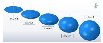
Fig. 7 The different cavity shapes studied by numerical simulation
