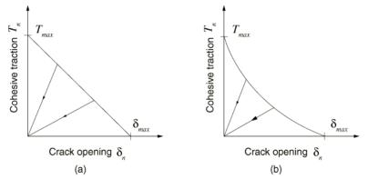
Fig. 1 Typical linear (a) and nonlinear (b) traction-separation response.
