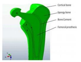
Fig. 2 Longitudinal section of the THP model.
