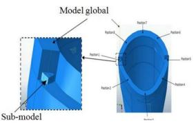
Fig. 6 Illustration of the submodel technique and the different positions of the defects (cavities)
