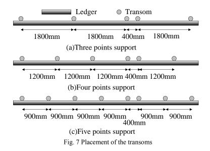
When the width of the rack column is 10000mm and each flange width of columns is 300mm, the clearance of the rack columns is 10000mm-300mm=9700mm. If the ledgers are tentatively placed every 1800mm, the number of the clearance division is 9700/1800=5.3. Therefore, seven ledgers are required and the interval of the ledgers is 9700mm/6=1617mm.
