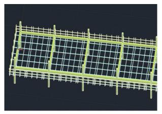
Fig. 8 Placement of the ledgers and the transoms
