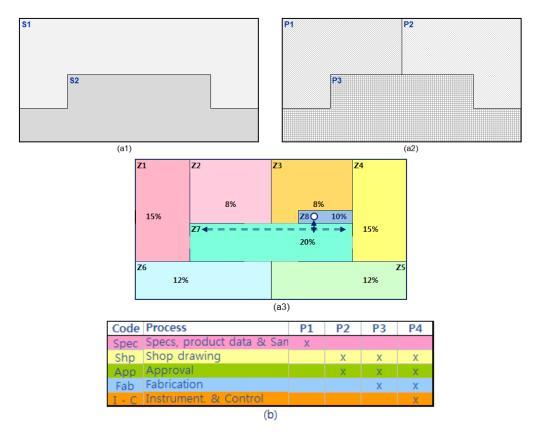
Fig. 3(a)-3(b) Chronographic model of scheduling for a building floor
