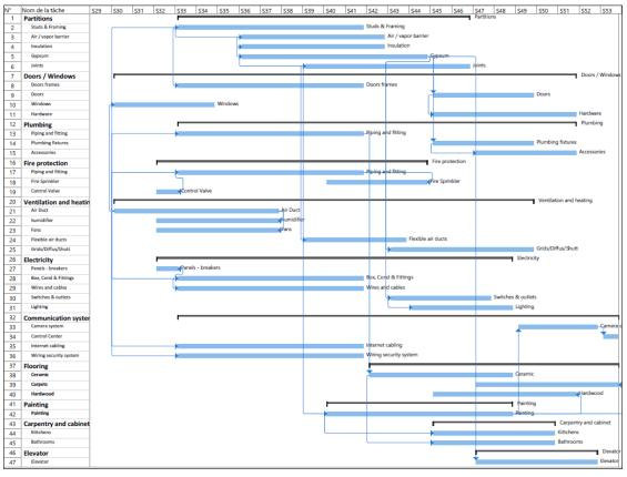
Fig. 1 Gantt-Precedence diagram scheduling for a building floor
