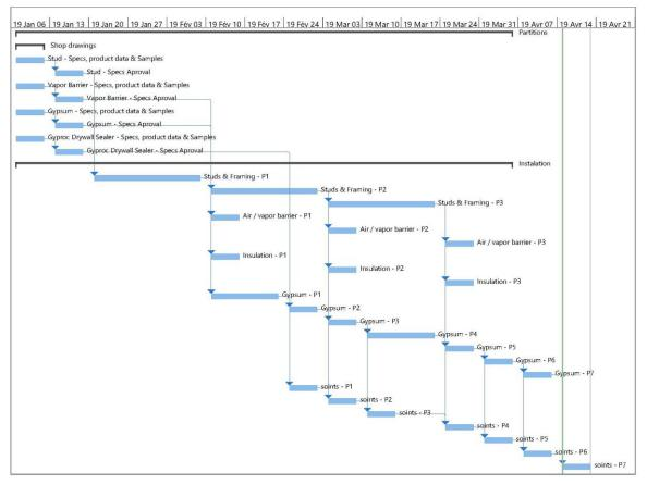
Fig. 5 Gantt-Precedence diagram for wall-partition planning
