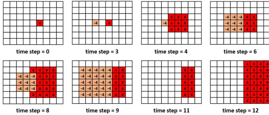
Fig. 8 Implementation of repellent propagation in a hazard-affected environment
