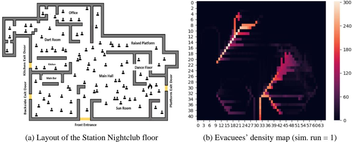
Fig. 17 Layout and evacuation pattern of the Rhode Island Station Nightclub fire incident
