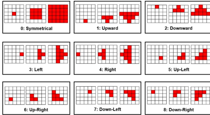
Fig. 4 Symmetrical and directional fire propagation at times 0,  $t_H$ , and  $2t_H$
