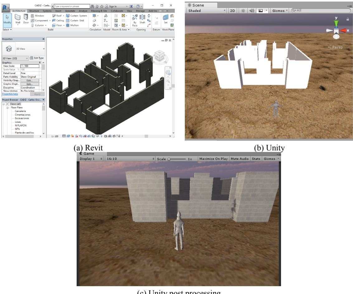
Fig. 3 Concrete block walls model in Revit and Unity
