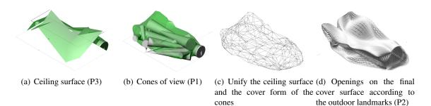
Fig. 11 Alternative study 2: Combine three algorithms based on three precedents (Fig. 6) in the following order: precedent P3 (a), then precedent P1 (b),(c); and at last precedent P2 (d)
