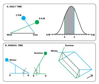
Fig. 1 Design mechanism of solar envelopes, generated from: A. daily time limits (Knowles 1980, p. 13) and B. annual time limits (Knowles 1981, p. 54)
