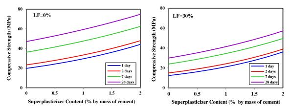
Fig. 8 Effect of Superplasticizer content on concrete compressive strength at various ages
