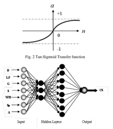
Fig. 3 Architecture of neural network model
