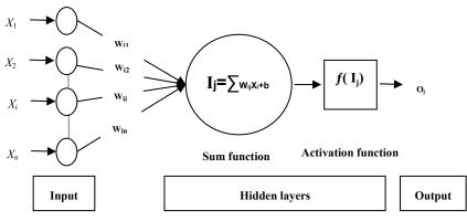
Fig. 1 Typical neural network architecture
