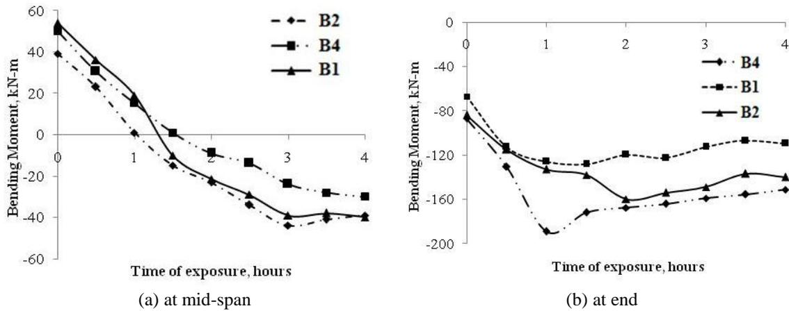
Fig. 12 Evolution of bending moment in beams
