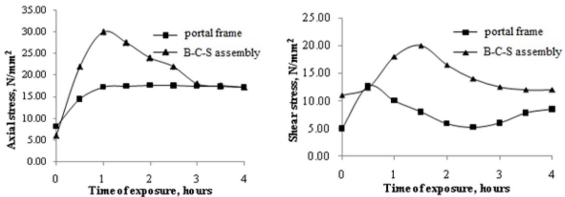
(a) Axial stress plot at beam-column joint
