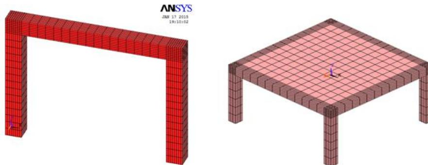
Fig. 5 Finite element model of RC frames exposed to fire
