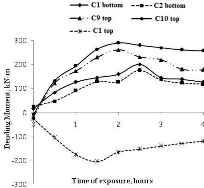
Fig. 11 Evolution of bending moment in columns of multi storeyed frame
