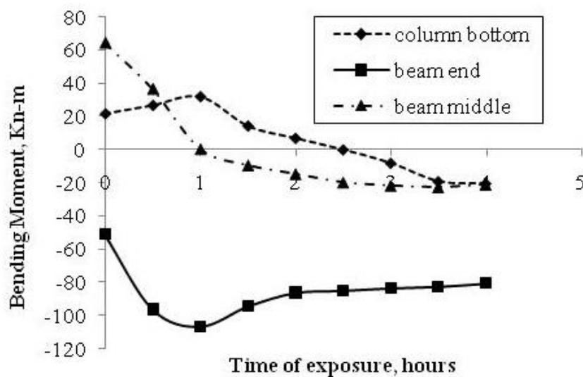
Fig. 10 Evolution of bending moments in portal frame subjected to fire
