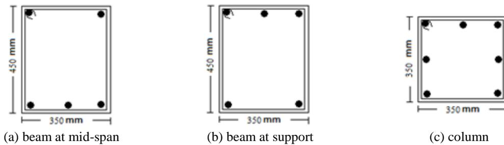
Fig. 4 Cross-section and reinforcement details of members of RC frames exposed to fire
