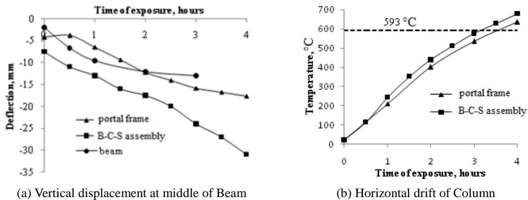
Fig. 8 Post fire deflection vs fire exposure time for various structures
