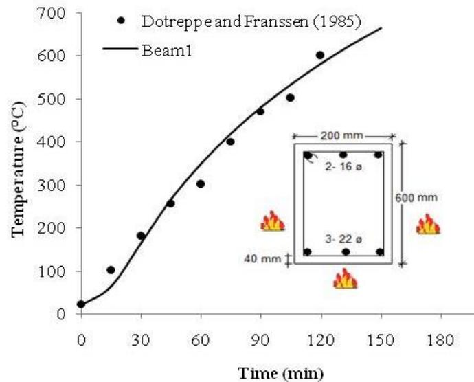
Fig. 3 Comparison of corner reinforcement temperature obtained from numerical analysis with test data (Dotrepe and Franssen 1985)
