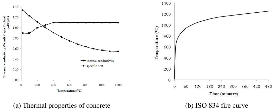
Fig. 1 Material properties and fire load for thermal analysis
