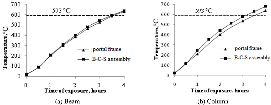
Fig. 7 Temperature variation in corner reinforcement with respect to time
