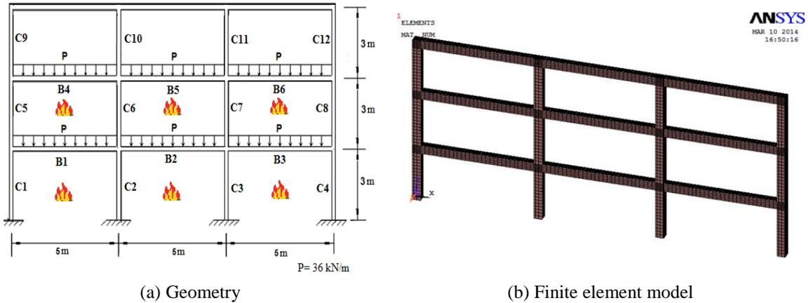
Fig. 6 Multi storey RC frame exposed to fire
