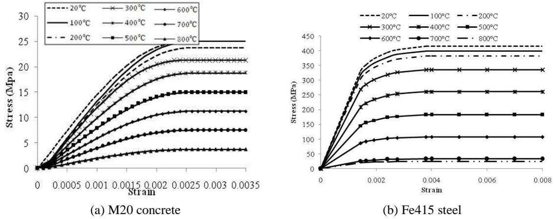
Fig. 2 Stress-strain curves of materials at various temperatures
