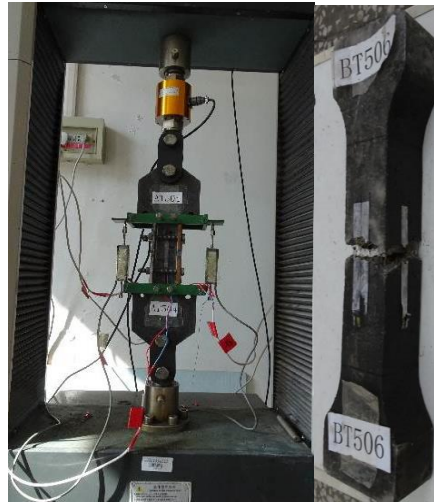
Fig. 16 Test setup and steel constraint
