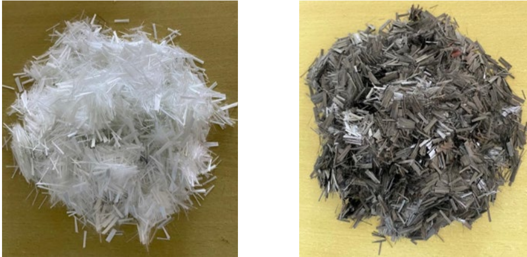
Fig. 1 Glass and carbon fiber used in this study
