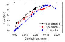
(a) Load- displacement of specimens with smooth interface
