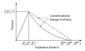
Fig. 2 Calculation diagram of cohesion model
