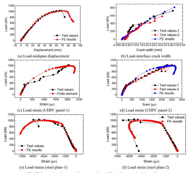
Fig. 22 Comparison between joint test results and finite element calculation values
