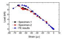
(b) Compressive strain on the upper side of smooth interface specimens
