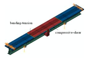
Fig. 21 Finite element model of joint test
