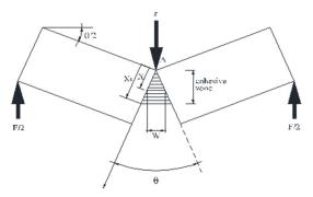
Fig. 15 Calculation diagram of initial separation distance
