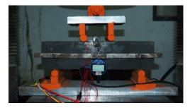
Fig. 8 Loading and measurement scheme of flexural test
