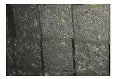
Fig. 7 Roughened surface of UHPC interface in flexural test
