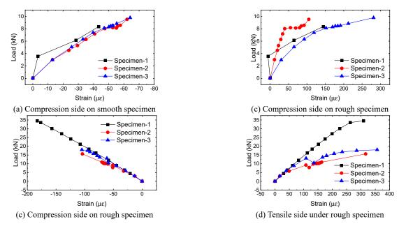
Fig. 11 Development curve of load-strain of flexural specimen
