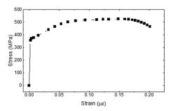
Fig. 6 Q345 steel plate compression stress-strain diagram
