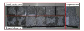
(a) Side view of failure surface of flexural test
