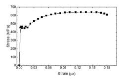
Fig. 5 Diagram of tensile stress-strain of reinforcement
