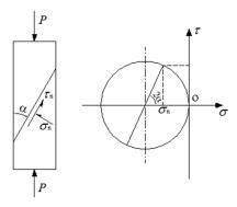
Fig. 19 Calculation of oblique shear specimen with Mohr-Coulomb circle
