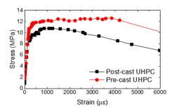
Fig. 4 Tensile stress-strain diagram of UHPC material
