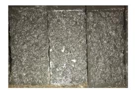
Fig. 16 Surface roughening of oblique shear specimen in rough interface group
