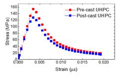
Fig. 3 UHPC Stress-strain diagram of UHPC material under pressure
