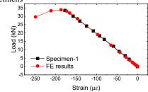
(d) Compressive strain on the upper side of rough interface specimens
