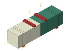
Fig. 12 Finite element model of bending test
