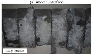
(b) rough interface Fig. 18 Failure of oblique shear specimen
