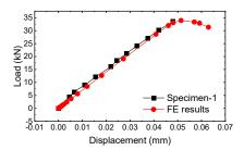
(c) Load- displacement of specimen with rough interface
