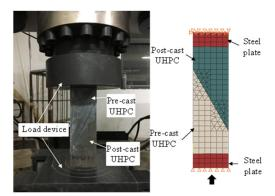
Fig. 20 Finite element model of oblique shear test
