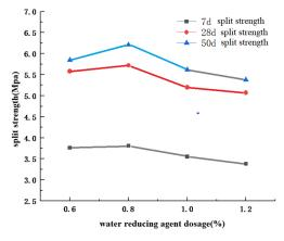
(b) Effect of different water-reducing agents on splitting tensile strength
