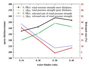
Fig. 5 The influence of different water-binder ratios and wind pressure on spray thickness and rebound
