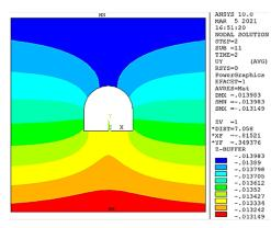
(b) Displacement in Y direction before support
