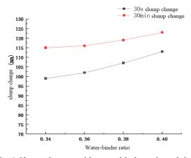
Fig. 1 Slump changes with water-binder ratio and time
