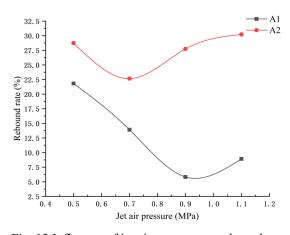
Fig. 13 Influence of jet air pressure on rebound rate
