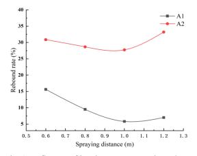
Fig. 15 Influence of jet air pressure on rebound rate
