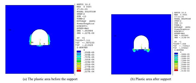
Fig. 22 Contrast cloud map of the plastic area before and after support
