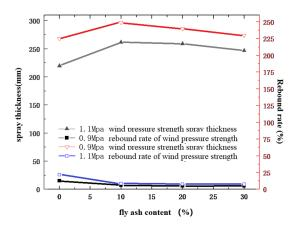
Fig. 6 The influence of different fly ash content and wind pressure on injection thickness and rebound
