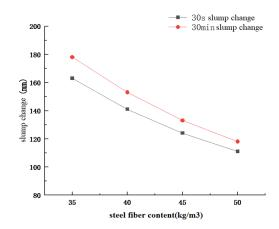
Fig. 4 Slump change with steel fibre content and time
