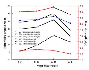
(a) Effect of different water binder ratios on flexural and compressive strength
