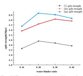
(b) Effect of different water binder ratio on splitting tensile strength
