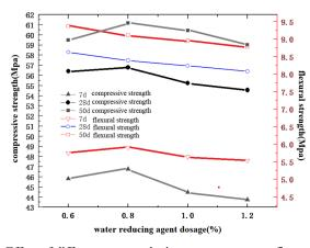
(a) Effect of different water reducing agent content on flexural and compressive strength
