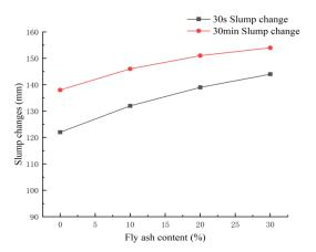
Fig. 2 Slump changes with fly ash content and time
