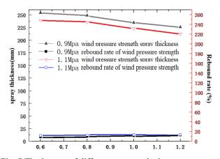
Fig. 7 The impact of different water-reducing agent content and wind pressure on spray thickness and rebound
