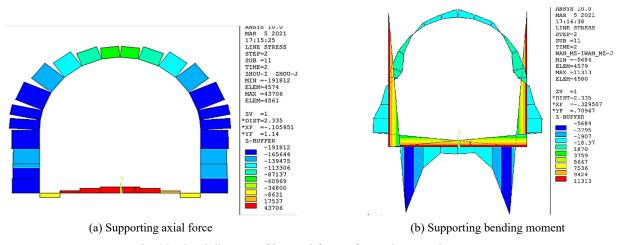
Fig. 23 Cloud diagram of internal force of tunnel supporting structure
