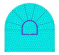
(b) Detailed finite element calculation model grid
