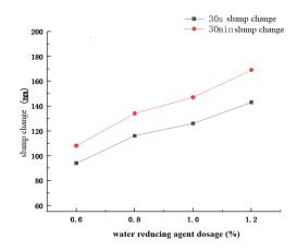
Fig. 3 Slump change with water reducing agent dosage and time
