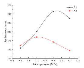
Fig. 14 Influence of jet wind pressure on the jet thickness
