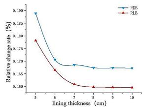
Fig. 19 Change curve of relative displacement convergence value
