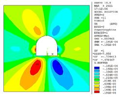
(c) Displacement in X direction after support
