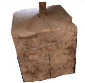
Fig. 18 Failure mode of the sample after bond test
