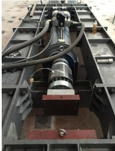
(a) Electric-hydraulic servo multi-function testing machine
