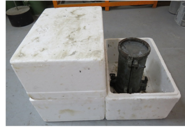
Fig. 3 Simulating the surface environment in the construction site by polystyrene boxes
