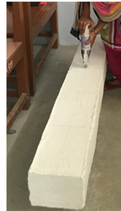
Fig. 10 Rebound hammer test on box beam
