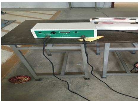
Fig. 9 Ultrasonic pulse velocity test on box beams
