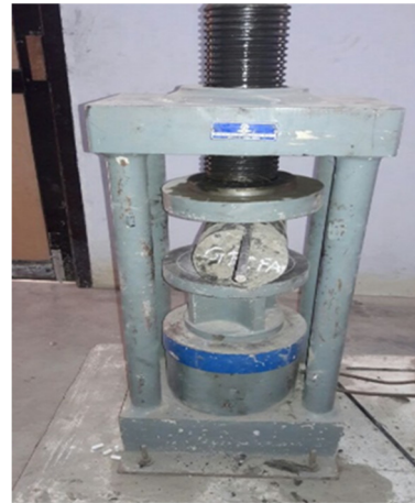
(b) Split tensile test on mortar cylinders
