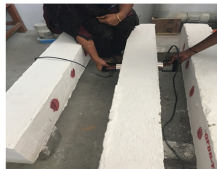
Fig. 9 Ultrasonic pulse velocity test on box beams
