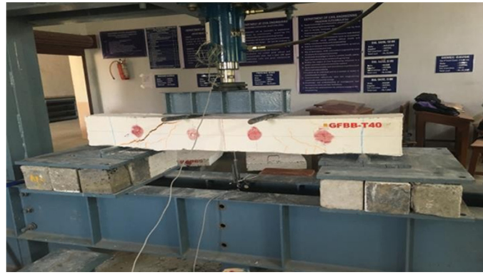
(a) Loading frame with hydraulic jack, load cell and LVDT
