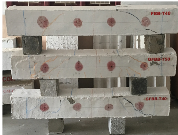
Fig. 19 Cracking characteristics of ferro-cement and ferro-geopolymer box beams under flexure
