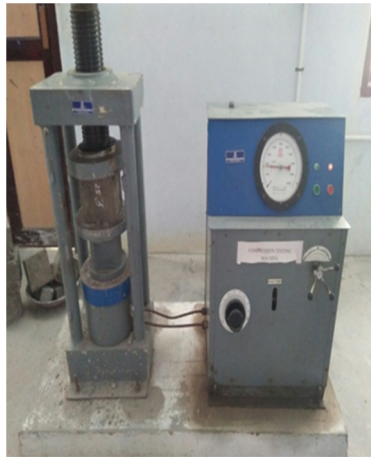
(a) Compressive strength test on mortar cubes
