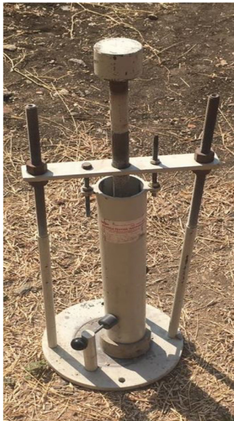
Fig. 8 Drop-weight impact test on mortar disc
