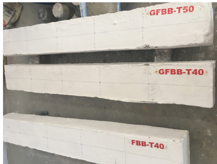
Fig. 5 Box beams after curing
