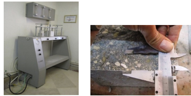
(a) Specimens under pressure (b) Measuring the depth of penetration by caliper
