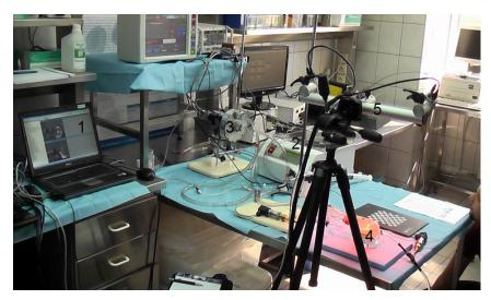
Fig. 2 An overview of the DIC experimental setup: 1 – PC and electronic system, 2 – tank and temperature stabilising system, 3 – centrifugal pump, 4 – pneumatic pump, and 5 – cameras
