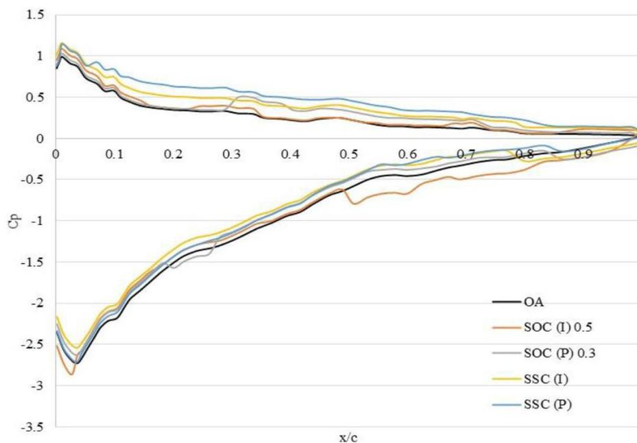
Fig. 6  $C_p$  distribution along the  $x/c$  chord location at  $10^\circ$  AOA
