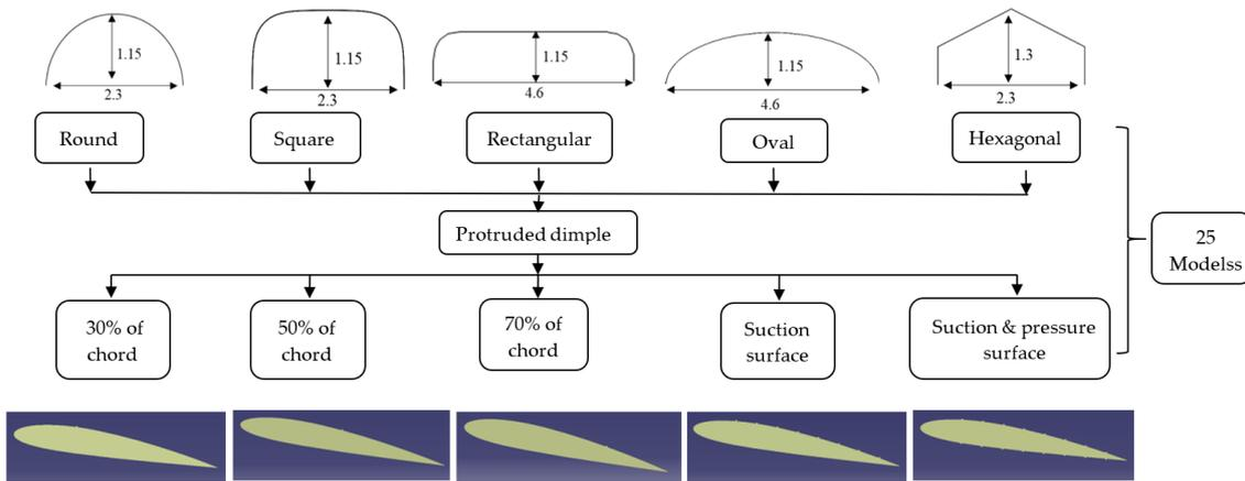
Fig. 2 Protruded cavity models
