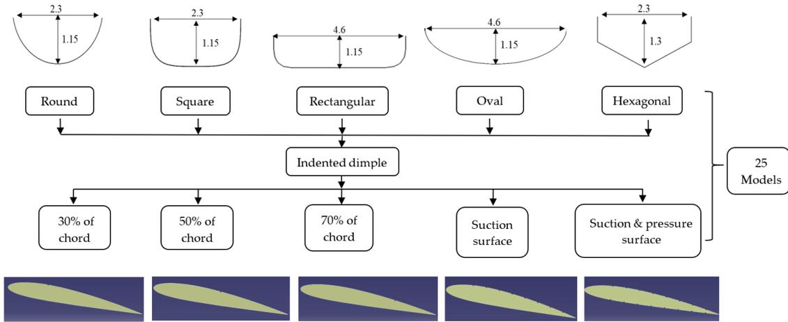
Fig. 1 Indented cavity models
