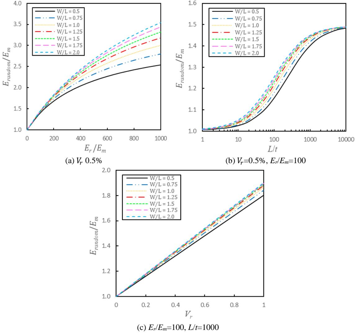
Fig. 2 Variations of elastic modulus for various filler geometry factors
