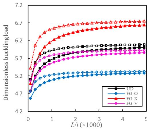
Fig. 7 Effect of  $L/t$  ratio on the dimensionless buckling of FG rGORC plates for various distribution types (Solid line:  $W/L=0.25$ , dashed line:  $W/L=1$ ,  $\Lambda_{rGO}=1\%$ ,  $l/h=0$ , CCCC)
