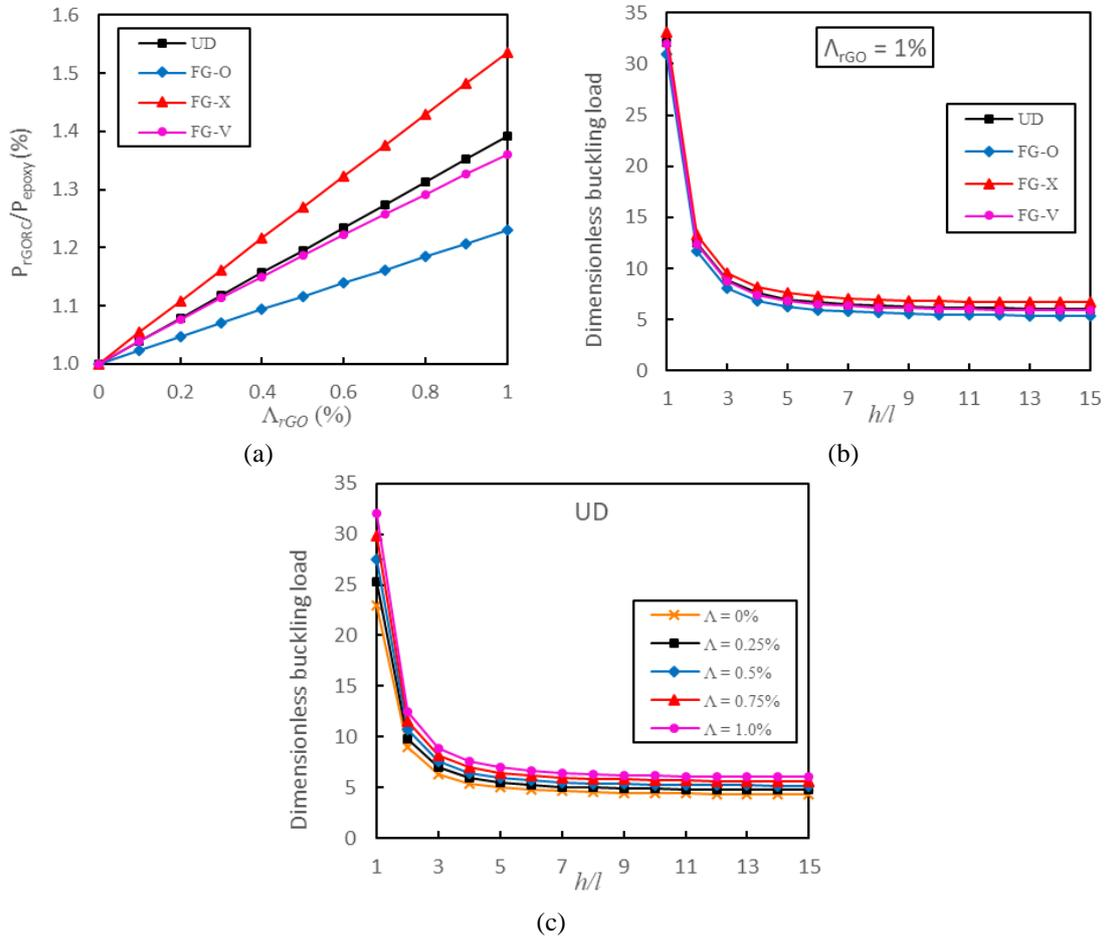
Fig. 6 Effect of rGO weight fraction on the buckling change (%) of FG rGORC plates for various distribution types (CCCC)
