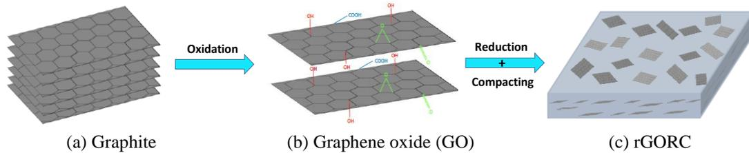
Fig. 1 Schematic illustration of the fabrication process for reduced graphene oxide reinforced composite (rGORC) plates
