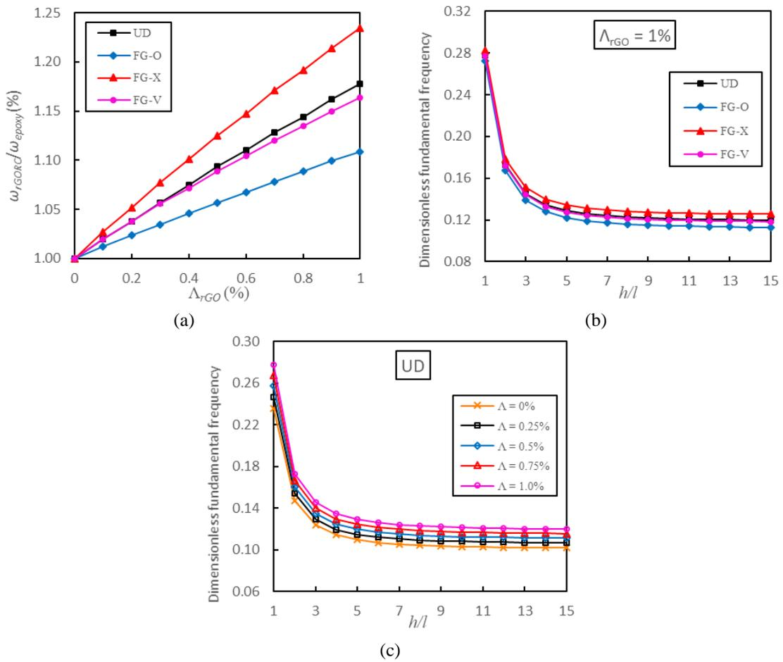
Fig. 4 Effect of rGO weight fraction on the fundamental frequency change (%) of FG rGORC plates for various distribution types (CCCC)
