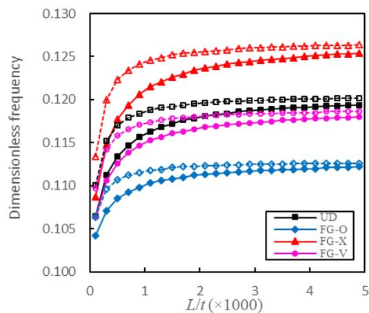
Fig. 5 Effect of  $L/t$  ratio on the dimensionless fundamental frequency of FG rGORC plates for various distribution types (Solid line:  $W/L=0.25$ , dashed line:  $W/L=1$ ,  $\Lambda_{rGO}=1\%$ ,  $l/h=0$ , CCCC)
