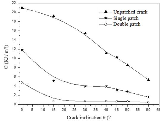
Fig. 16 Comparison of the fracture energy between patched and unpatched cracks in mixed mode
