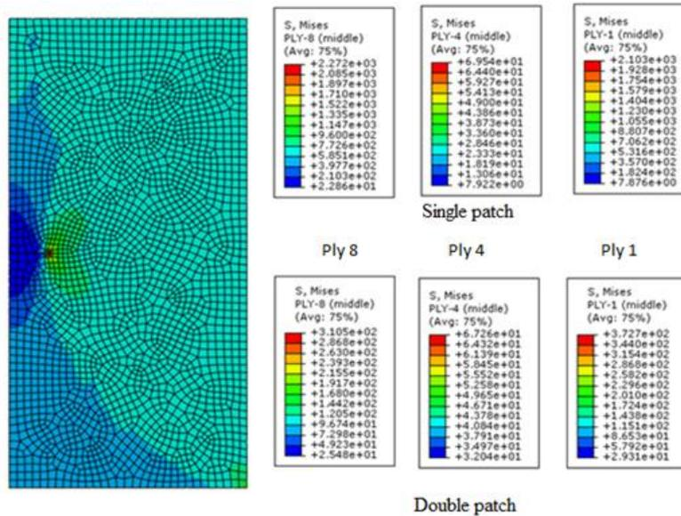
Fig. 10 Contour of Von Mises stresses (MPa) in the various layers of the plate
