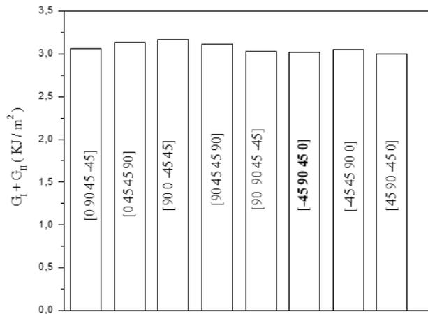
Fig. 19 Effect of plies orientation of the single patch on the GI+GII values ( $\theta = 45^\circ$ ,  $2a = 50$  mm)
