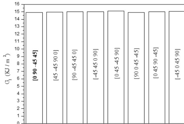
Fig. 7 Effect of plies orientation of the patch on the GI values
