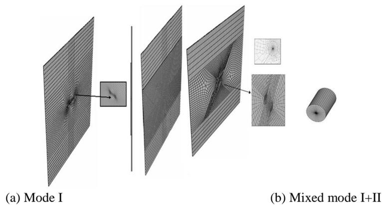
Fig. 2 Typical mesh model of the plate, patch and near the crack tip in pure mode I and mixed mode I+II
