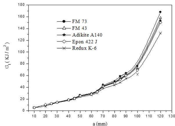
Fig. 11  $G_I$  vs crack length for different adhesives
