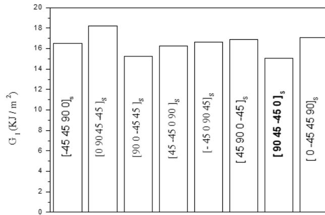
Fig. 6 Effect of plies orientation of the repaired plate on the GI values
