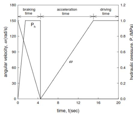
Fig. 7 The operation conditions used in transient thermoelastic analysis
