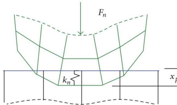
Fig. 4 The contact stiffness between two contact parts (ANSYS 14 user’s manual)
