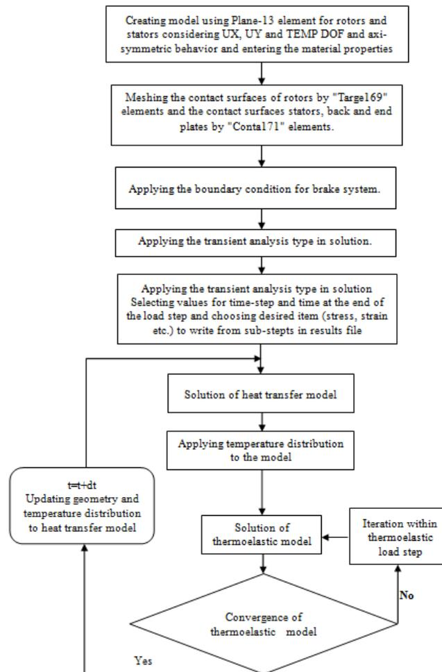
Fig. 5 Procedure of the transient thermoelastic analysis
