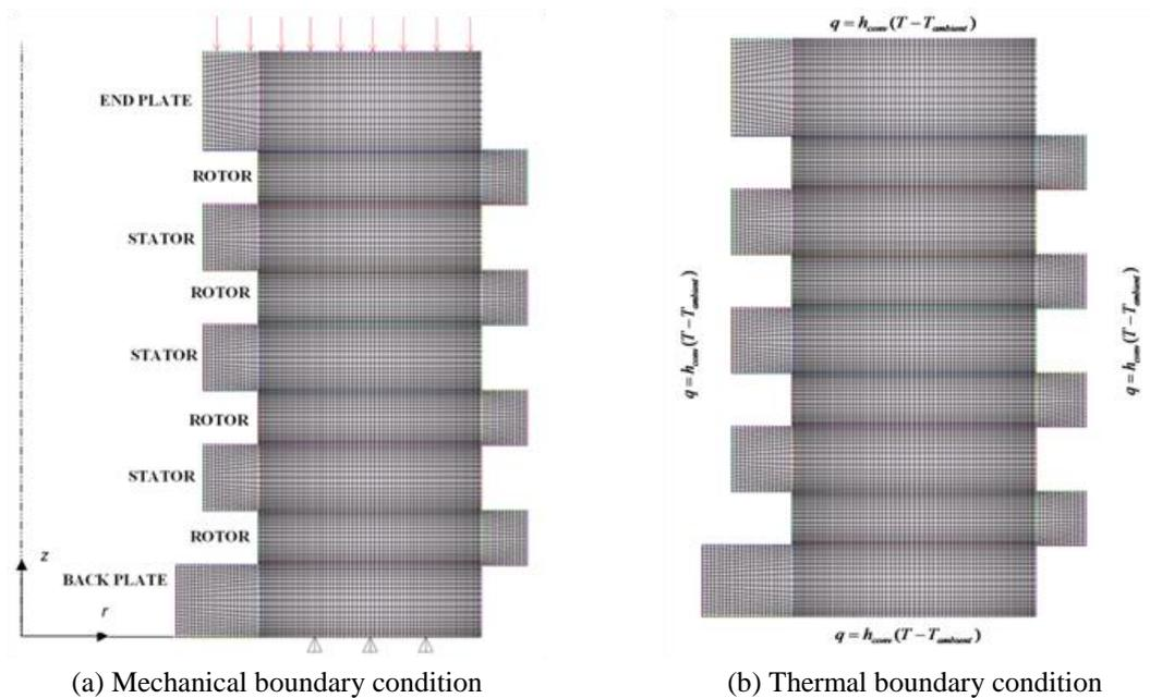
Fig. 2 The finite element model of multidisc brake system
