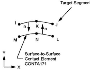
Fig. 3 Geometry of Conta171 and Targe169 elements (ANSYS 14 user’s manual)
