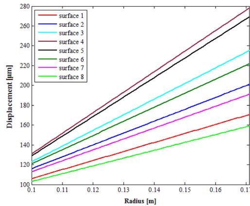
Fig. 11 Maximum displacement in different discs surfaces versus radius
