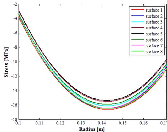
Fig. 12 Maximum stresses in different discs surfaces versus radius
