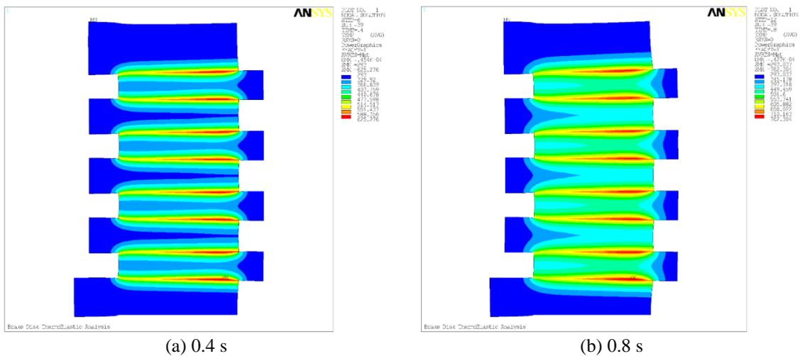
Fig. 9 Temperature contours of multidisc brake system obtained at selected time intervals ( $^{\circ}\text{K}$ )
