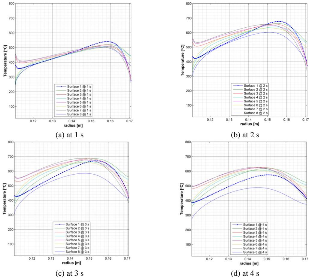
Fig. 8 The distributions of temperature on all contact surfaces at selected time intervals
