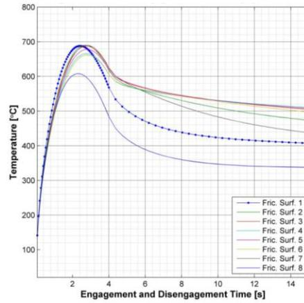
Fig. 10 Maximum temperature in different discs surfaces versus time
