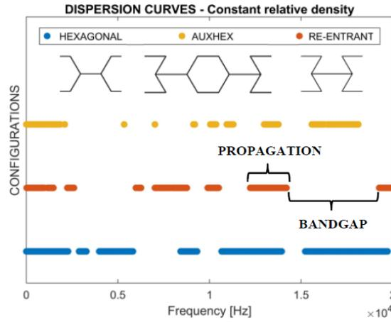
Fig. 13 Dispersion curve of the three topologies considered for the comparison
