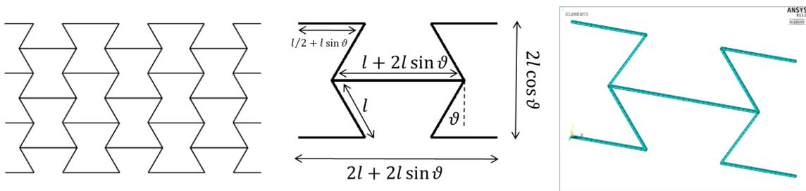
Fig. 7 Re-entrant unit cell (left) and example core (right)
