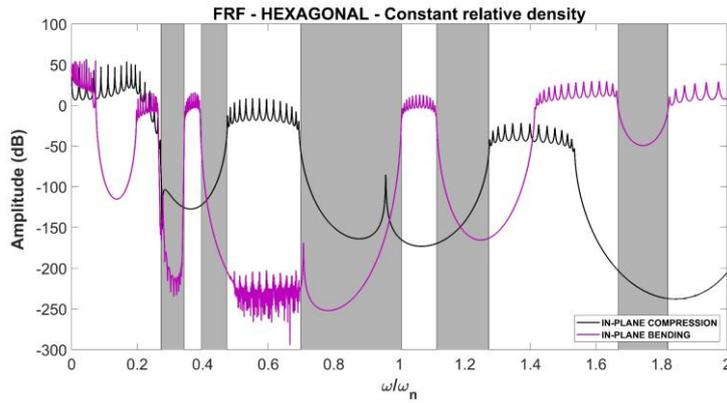
Fig. 5 FRF plot for Hexagonal topology
