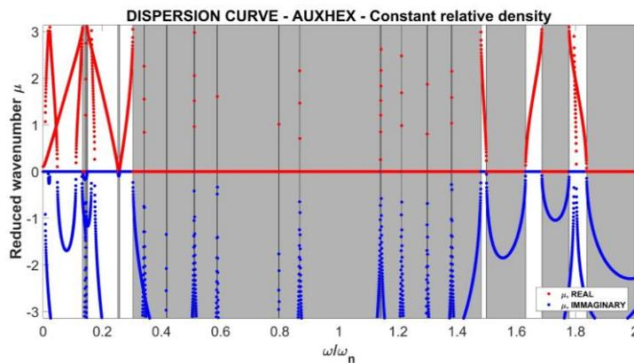
Fig. 12 Dispersion curve for AUXHEX topology
