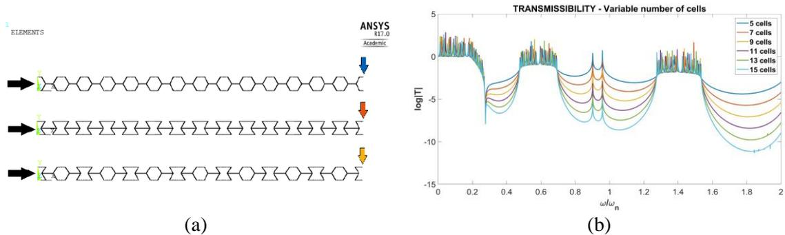
Fig. 2 (a) Analysed truss structures with input force (black arrows) and output readings (coloured arrows) and (b) In-plane compression 1D FRF for increasing number of cells
