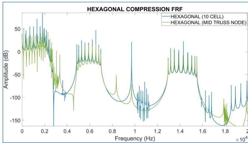
Fig. 20 Nodal output at the middle of the new truss versus the output at the end of a hexagonal core truss
