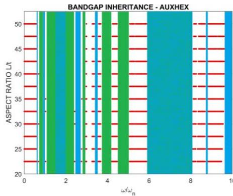
Fig. 18 Parametric dispersion curve for the AUXHEX configuration. The inherited bandgaps are shown in blue (from Hexagonal) and green (from Re-entrant)
