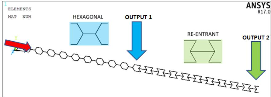
Fig. 19 New truss structure (10 hexagonal + 10 re-entrant unit cells)
