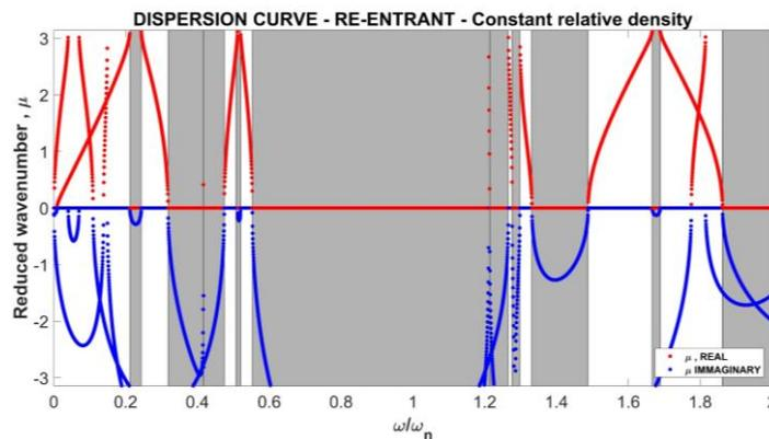
Fig. 9 Dispersion curve for Re-entrant topology
