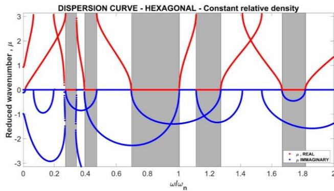
Fig. 6 Dispersion curve for Hexagonal topology
