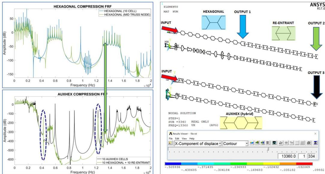
Fig. 22 Deformed shape of the new truss structure when solicited at 13360 Hz
