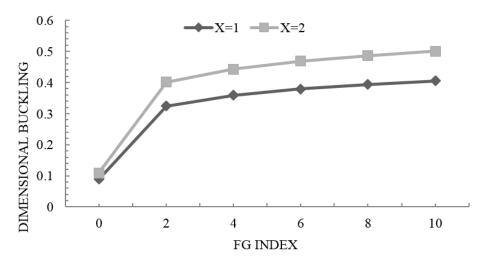
Fig. 9 Change of dimensional buckling versus FG material's parameter in different nonlinear load factor ( $\chi$ ) in  $\beta = 1$ ,  $l_x = 10 nm$  and  $\mu = 1 nm$
