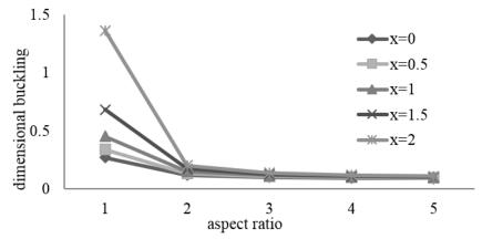
Fig. 6 The effect of different aspect ratio on the dimensional buckling load for ssss B.C in different linear load factor ( $\mu = 1 nm$ ,  $l_x = 10 nm$  and k = 2)
