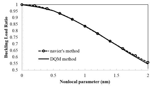
Fig. 3 Change of buckling load ratio with the nonlocal parameter for different load factors ( $l_x = 10 \text{ nm}$ )
