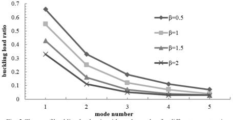
Fig. 5 Change of buckling load ratio with mode number for different aspect ratio
