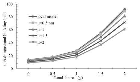
Fig. 4 The effect of different loading condition on the non-dimensional buckling load for ssss nanoplates ( $\beta$ =0.5 and  $l_x = 10$ )
