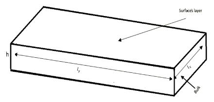
Fig. 1 Schematic view of functionally graded nanoplate
