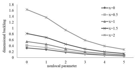
Fig. 7 The effect of different nonlocal parameter on the dimensional buckling load for ssss B.C in different linear load factor ( $\beta = 1$ ,  $l_x = 10 \text{ nm}$  and k = 2)
