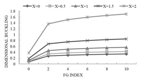
Fig. 8 Change of dimensional buckling versus FG material's parameter in different linear load factor ( $\chi$ ) in  $\beta = 1$ ,  $l_x = 10 nm$  and  $\mu = 1 nm$
