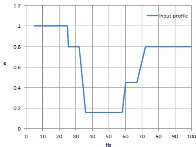
Fig. 4 Input profile for the qualification run (manual notching), x-axis
