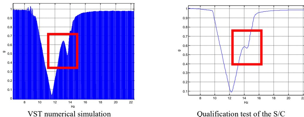
Fig. 6 S/C pilot along the excitation (x-axis); zoom on primary notching
