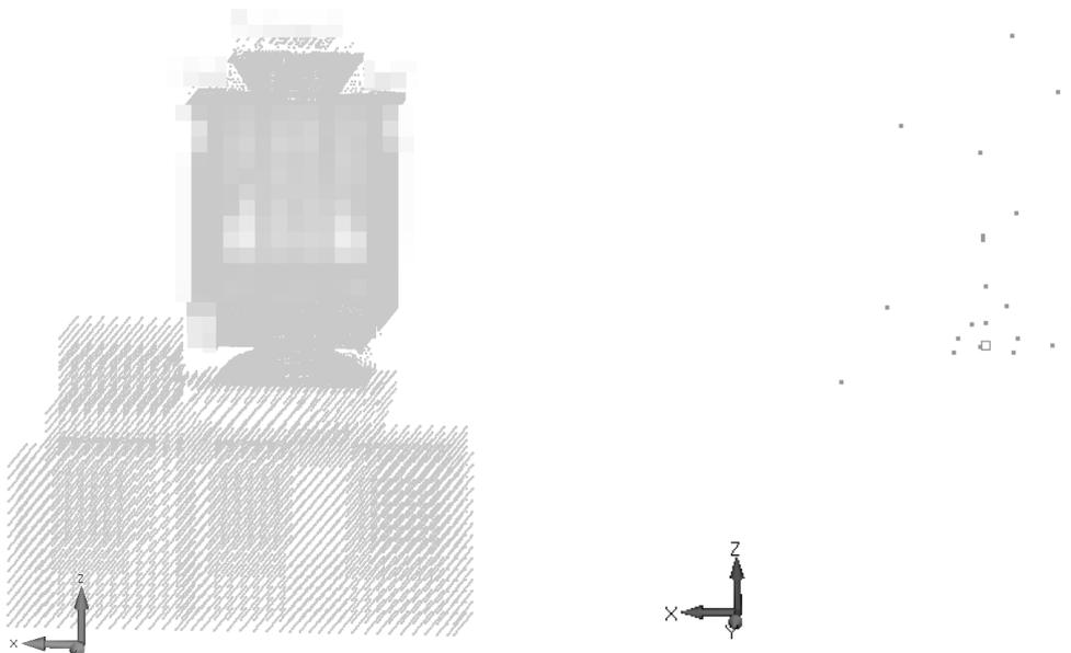
Fig. 3 VST assembly FE nodes before and after the reduction, from left to right
