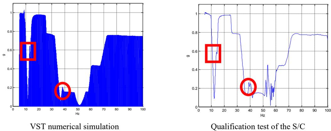
Fig. 5 S/C pilot along the excitation (x-axis)
