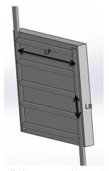
Fig. 2 Radiative Heat Exchanger (RHX)
