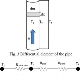
Fig. 4 Thermal model of the pipe
