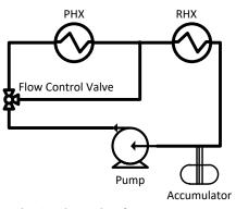
Fig. 1 Schematic of a MPFL system
