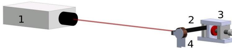
Fig. 2 Experimental setup for free vibrations of cantilever beams: laser doppler vibrometer (1), cantilever beam specimen (2), clamping with force monitoring (3) and a harpin coil for inductive excitation (4)
