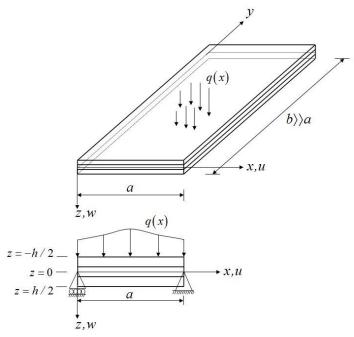
Fig. 1 Geometry of a plate strip in cylindrical bending
