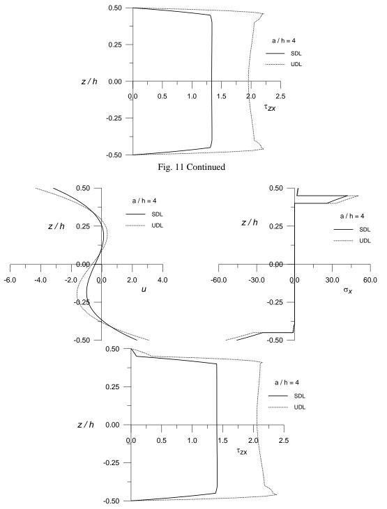
Fig. 12 Through thickness variation of in-plane displacement ( $\overline{u}$ ) at (x=0, z), in-plane normal stress ( $\overline{\sigma}_x$ ) at (x=a/2, z) and transverse shear stress ( $\overline{\tau}_{zx}$ ) at (x=0, z) for five layered ( $0^0/90^0/\text{core}/0^0/90^0$ ) antisymmetric sandwich plates subjected to sinusoidally distributed load (SDL) and uniformly distributed load (UDL)
