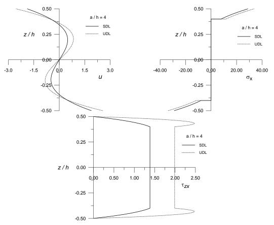
Fig. 10 Through thickness variation of in-plane displacement ( $\overline{u}$ ) at (x=0, z), in-plane normal stress ( $\overline{\sigma}_x$ ) at (x=a/2, z) and transverse shear stress ( $\overline{\tau}_{zx}$ ) at (x=0, z) for three layered ( $0^0$ /core/ $0^0$ ) symmetric sandwich plates subjected to sinusoidally distributed load (SDL) and uniformly distributed load (UDL)
