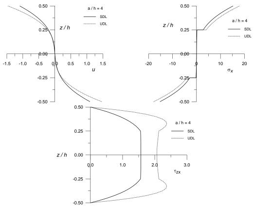
Fig. 7 Through thickness variation of in-plane displacement ( $\overline{u}$ ) at (x = 0, z), in-plane normal stress ( $\overline{\sigma}_x$ ) at (x=a/2, z) and transverse shear stress ( $\overline{\tau}_{zx}$ ) at (x = 0, z) for four layered ( $0^0/90^0/90^0/0^0$ ) symmetric laminated composite plates subjected to sinusoidally distributed load (SDL) and uniformly distributed load (UDL)
