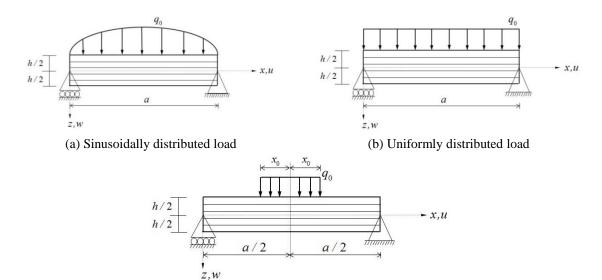
(c) Patch load Fig. 2 Laminated plates subjected various static loadings
