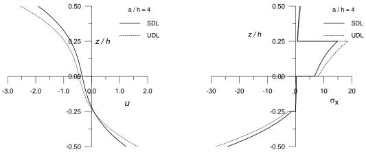
Fig. 5 Through thickness variation of in-plane displacement ( $\overline{u}$ ) at (x = 0, z), in-plane normal stress ( $\overline{\sigma}_x$ ) at (x=a/2, z) and transverse shear stress ( $\overline{\tau}_{zx}$ ) at (x = 0, z) for four layered ( $0^0/90^0/0^0/90^0$ ) antisymmetric laminated composite plates subjected to sinusoidally distributed load (SDL) and uniformly distributed load (UDL)
