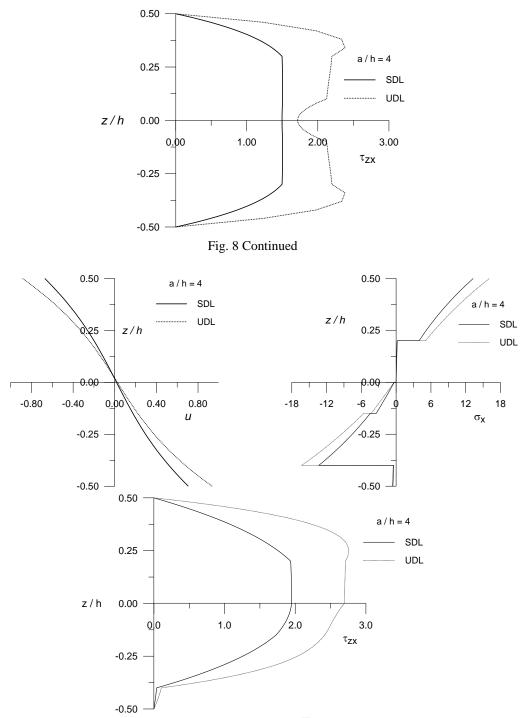
Fig. 9 Through thickness variation of in-plane displacement ( $\overline{u}$ ) at (x = 0, z), in-plane normal stress ( $\overline{\sigma}_x$ ) at (x=a/2, z) and transverse shear stress ( $\overline{\tau}_{zx}$ ) at (x=0, z) for five layered (90<sup>0</sup>/0<sup>0</sup>/90<sup>0</sup>/0<sup>0</sup>) arbitrary laminated composite plates subjected to sinusoidally distributed load (SDL) and uniformly distributed load (UDL)
