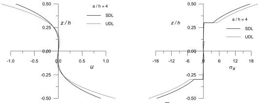
Fig. 8 Through thickness variation of in-plane displacement ( $\overline{u}$ ) at (x=0, z), in-plane normal stress ( $\overline{\sigma}_x$ ) at (x=a/2, z) and transverse shear stress ( $\overline{\tau}_{zx}$ ) at (x=0, z) for five layered ( $0^0/90^0/0^0/90^0/0^0$ ) sy mmetric laminated composite plates subjected to sinusoidally distributed load (SDL) and uniformly distributed load (UDL)
