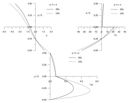
Fig. 4 Through thickness variation of in-plane displacement ( $\overline{u}$ ) at (x=0, z), in-plane normal stress ( $\overline{\sigma}_x$ ) at (x=a/2, z) and transverse shear stress ( $\overline{\tau}_{zx}$ ) at (x=0, z) for two layered ( $0^0/90^0$ ) antisymmetric laminated composite plates subjected to sinusoidally distributed load (SDL) and uniformly distributed load (UDL)
