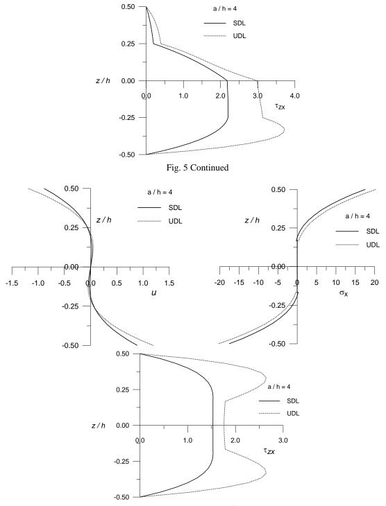
Fig. 6 Through thickness variation of in-plane displacement ( $\overline{u}$ ) at (x = 0, z), in-plane normal stress ( $\overline{\sigma}_x$ ) at (x=a/2, z) and transverse shear stress ( $\overline{\tau}_{zx}$ ) at (x = 0, z) for three layered ( $0^0/90^0/0^0$ ) symmetric laminated composite plates subjected to sinusoidally distributed load (SDL) and uniformly distributed load (UDL)
