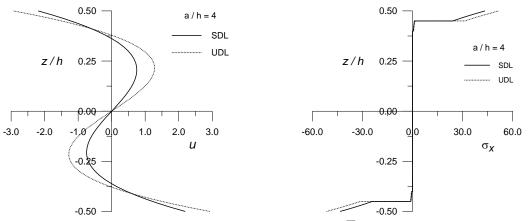
Fig. 11 Through thickness variation of in-plane displacement ( $\overline{u}$ ) at (x=0, z), in-plane normal str ess ( $\overline{\sigma}_x$ ) at (x=a/2, z) and transverse shear stress ( $\overline{\tau}_{zx}$ ) at (x=0, z) for five layered ( $0^0/90^0$ /core  $/90^0/0^0$ ) symmetric sandwich plates subjected to sinusoidally distributed load (SDL) and uniformly distributed load (UDL)
