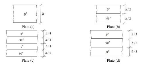
Fig. 3 Laminate configurations
