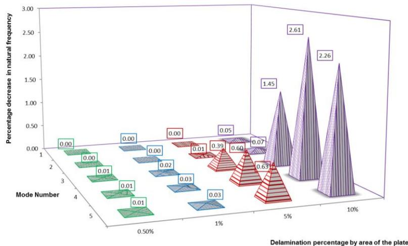
Fig. 6 Shift in natural frequency for one way simply supported panel: delamination position 2
