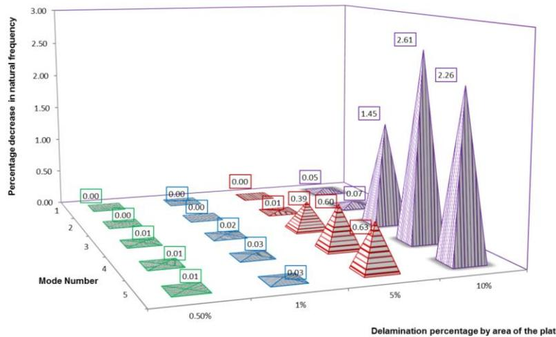
Fig. 5 Shift in natural frequency for one way clamped panel: delamination position 2
