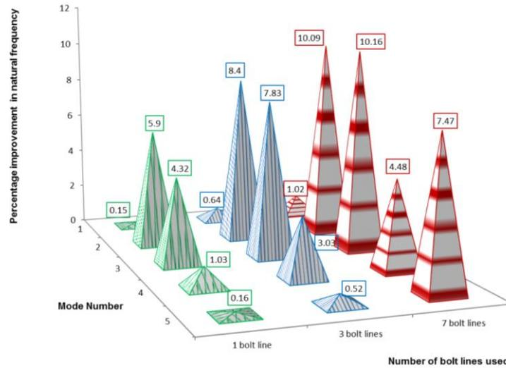
Fig. 8 Natural frequency improvement due to fastening the delaminated region in C-C-C-C plate
