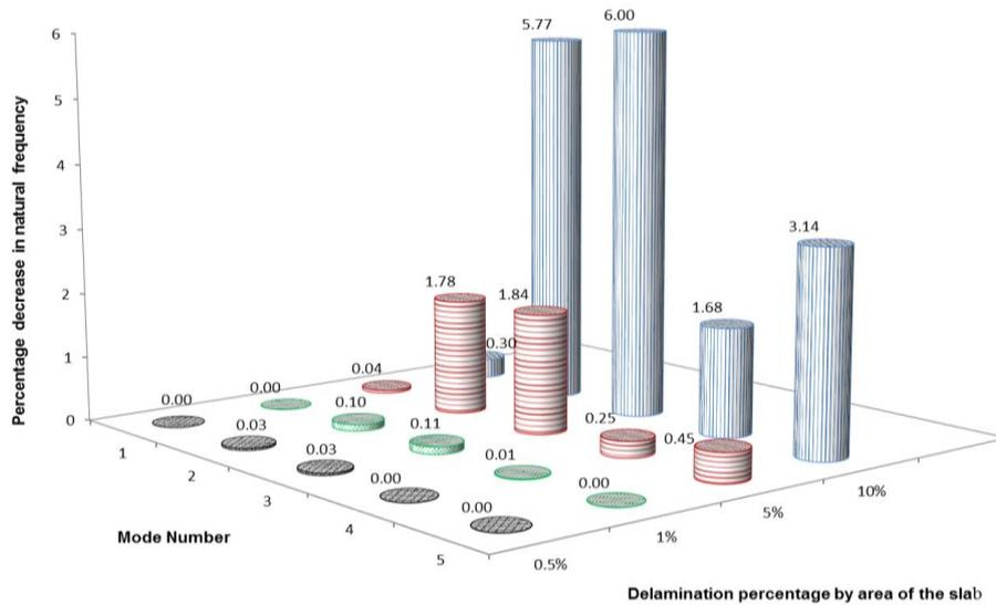
Fig. 3 Shift in natural frequency for two way clamped panel: delamination position 3
