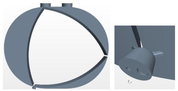
Fig. 1 Simplified Wankel rotor geometry. The details of the jet ignition device are not optimized to deliver the best performances on the specific geometry
