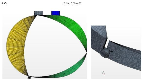
Fig. 2 Computational grid. The details of the computational mesh are not optimized to deliver the best simulation results on the specific geometry
