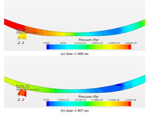
Fig. 3 Pressure evolution during combustion and expansion. As shown in the hydrogen profile of Figure 5, combustion starts in the pre-chamber at the spark plug electrodes (a), then extends to the entire pre-chamber (b)
