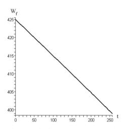
Fig. 1 Fuel of the CP-1 airplane as it climbs at 20°, at the speed of 25 m/s, up to 2190 m
