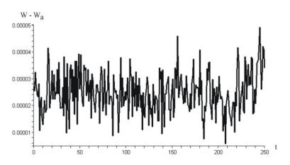
Fig. 5 Difference between the exact value of the weight W(t) and the approximate value  $W_a(t)$ , for the trajectory of the CP-1 at 20° with the speed of 25 m/s
