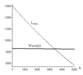
Fig. 3 Wcos( $\theta$ ), represented by the solid line, and  $L_{\text{max}}$ , represented by the dotted line, as a function of the altitude, for the climbing airplane CP-1 at 20°, with a constant speed of 25 m/s
