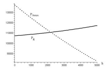
Fig. 2 Required power  $P_R$  and maximum available power  $P_{Amax}$  as a function of altitude h, for the climbing airplane CP-1 at 20°, with a constant speed of 25 m/s
