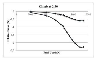
Fig. 4 Relative error in the approximation of the amount of fuel in % for a  $2.5^{\circ}$  climb-angle of the Hercules-Like airplane, in terms of the total fuel used in the trajectory. The curve with the square markers and that with the round markers correspond respectively to the one-step and the two-step linear approximation.
