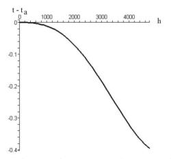
Fig. 8 The error  $t(h)-t_a(h)$  as a function of the altitude *h*, for a climb of the CP-1 airplane at 10°, climbing from sea level with a speed of 25 m/s, up to 4748 m
