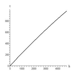
Fig. 7 Time as a function of altitude, for the CP-1 airplane climbing at  $10^{\circ}$ , starting at the speed of 25 m/s, up to 4748 m
