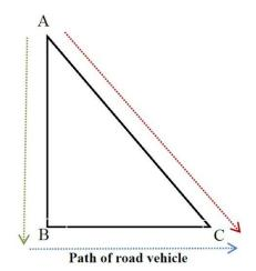
Fig. 3 Different travel distance between the drone and road vehicles with the same starting point and ending point
