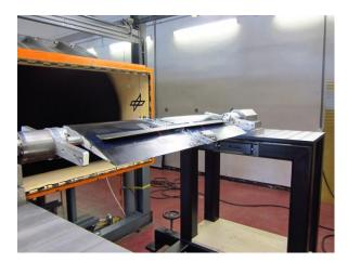
Fig. 3 Passive back-flow flap model in the 1MG at 50 m/s. Flow is from left to right
