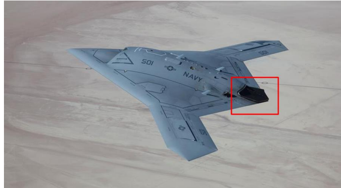
Fig. 1 Aircraft with embedded jet propulsion system and downstream ‘deck’
