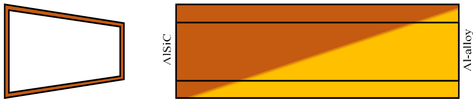
Fig. 3 Axial material grading: AlSiC at left and Al-alloy to the right
