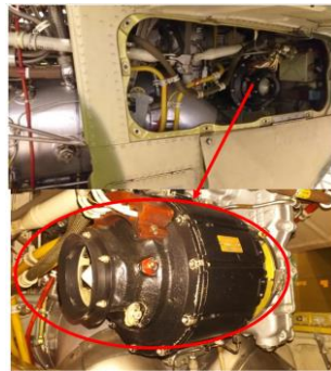
Fig. 9 M-28 B aircraft generator
