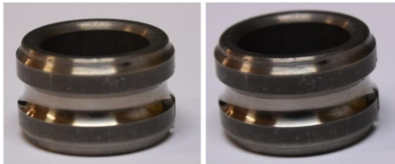
Fig. 3 Views of the inner ring of the starter ball bearing
