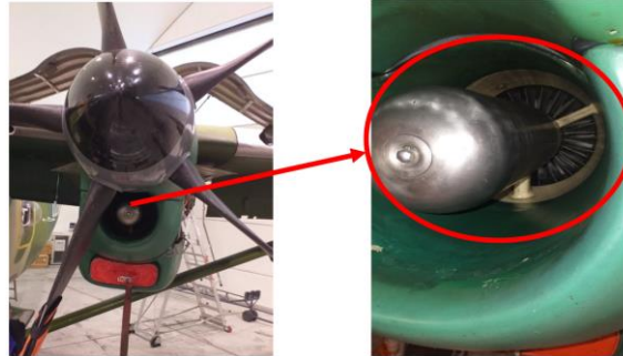
Fig. 8 M-28 B aircraft starter
