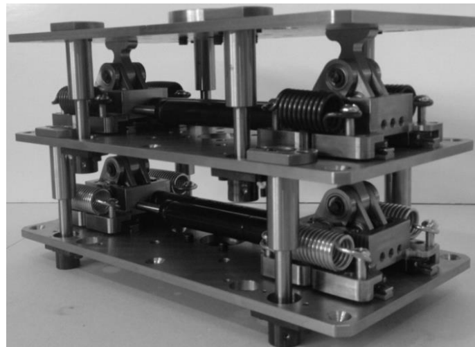
Fig. 8 Complete two layer prototype with 1,068 N/m (top layer) and 4,553 N/m (bottom layer) springs
