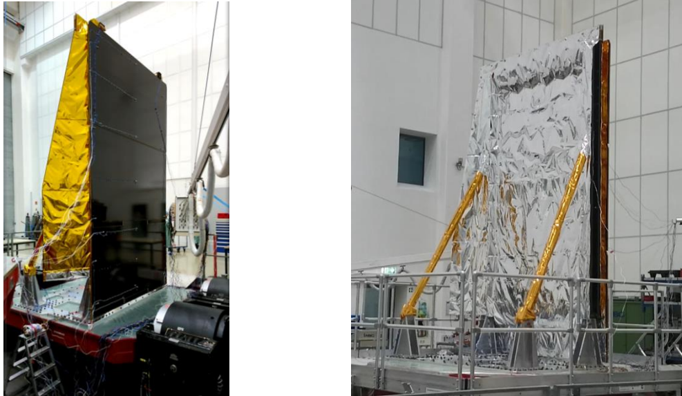
Fig. 9 SSH on the shaker: (a) excitation in X direction and (b) in Z direction
