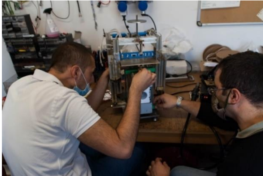
Fig. 9 Photo of the CTP installation on the Thrust Balance
