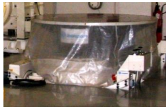
Fig. 5 Intespace 320 kN bi-shaker in empty vertical configuration
