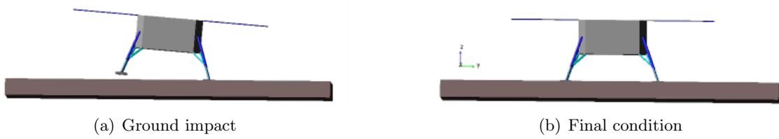
Fig. 9 2D landing of the lander with P control system.
