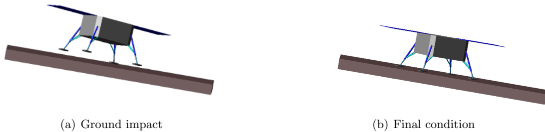
Fig. 14 3D landing of the lander with P control system.
