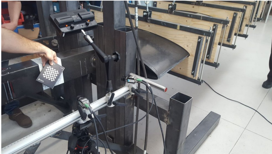
Figure 4 Calibration of Q-400 DIC system in CFM hangar
