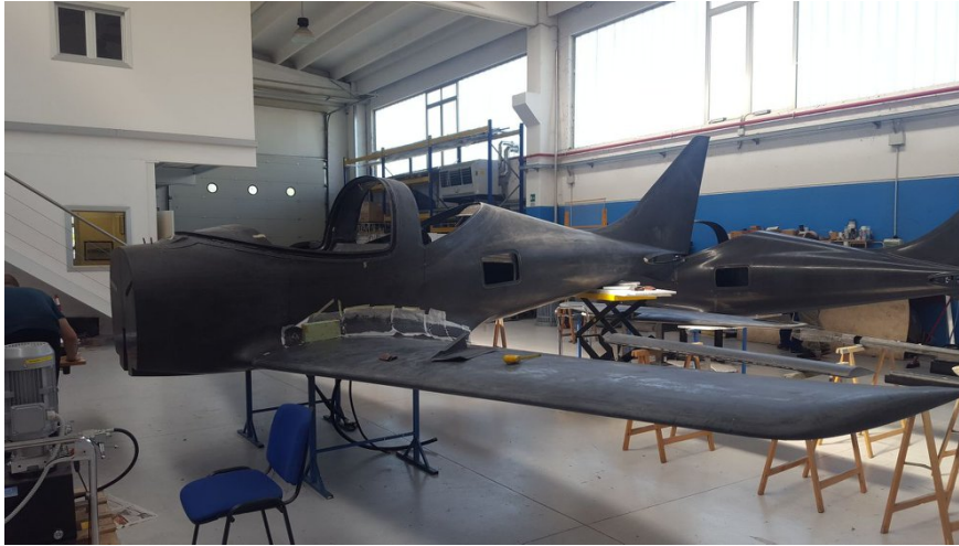
Figure 1 Primary composite structure of CFM Air Dardo Aspect
